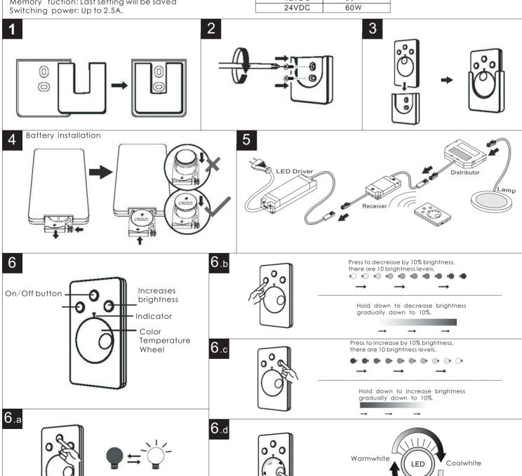
Rotate to select the desired color temperature
