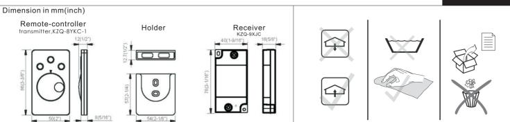
working frequency: 2.4GHz power:CR2032(3V) button lithium battery Remote range:≤15m
