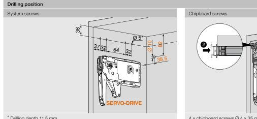
\* Drilling depth 11.5 mm
