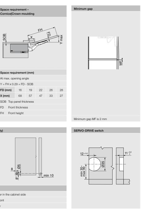
At max. opening angle Y = FH x 0.29 + FD - SOB FD (mm) 16 19 X (mm) SOB Top panel thickness FD Front thickness FH Front height
