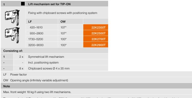
The power factor (LF) can be increased by 50% if you use a third lift mechanism. We recommend a third lift mechanism for wide cabinets. This will prevent the front from sagging when open.
