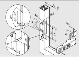
\* When changing material thickness, adjust the assembly dimensions accordingly
