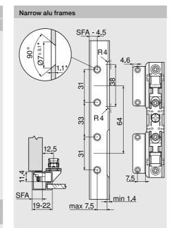
For frame width 19 mm, an SFA of 11–18 mm is possible.
