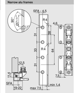
For frame width 19 mm, an SFA of 11-18 mm is possible.
