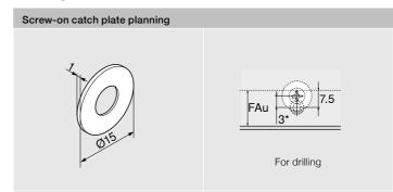
\* For the screw-on catch plate we recommend positioning the catch plate 3 mm away from TIP-ON. FAu Bottom front overlay
