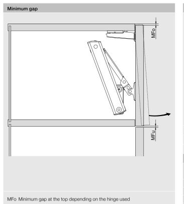
Overlay application ŝ 2. 66.5 TB 3-7 F Gap FA Front overlay TB Drilling distance Drilling distance TB Front overlay FA (mm) Q 5 6 7 8 9 10 11 12 13 14 15 16 17 18 0 3 4 5 6 7 3 3 4 5 6 7 3 4 5 6 7 6 9 3 4 5 6 7 MD Mounting plate spacing (mm)
