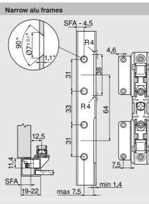
For frame width 19 mm, an SFA of 11-18 mm is possible.
