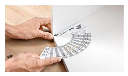
When it comes to mounting the fronts, we have further assembly devices in our range. These include our drilling templates for hinges, which ensure that the drilling positions on the front match those on the cabinet precisely. This results in hinges working perfectly – the doors close beautifully and the gap layout is faultless.
