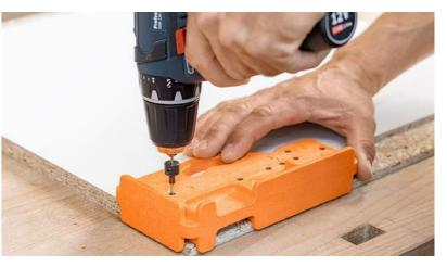
Drilling the holes is a process that requires the utmost in precision. With our drilling templates, marking and pre-drilling the fixing positions for the cabinet profiles couldn't be easier. You'll have the components perfectly prepared for assembly in no time.
